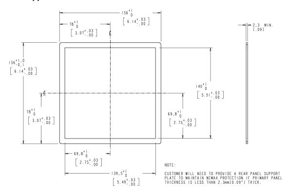
**Figure 3-2 Rear Panel Support Plate Dimensions**
